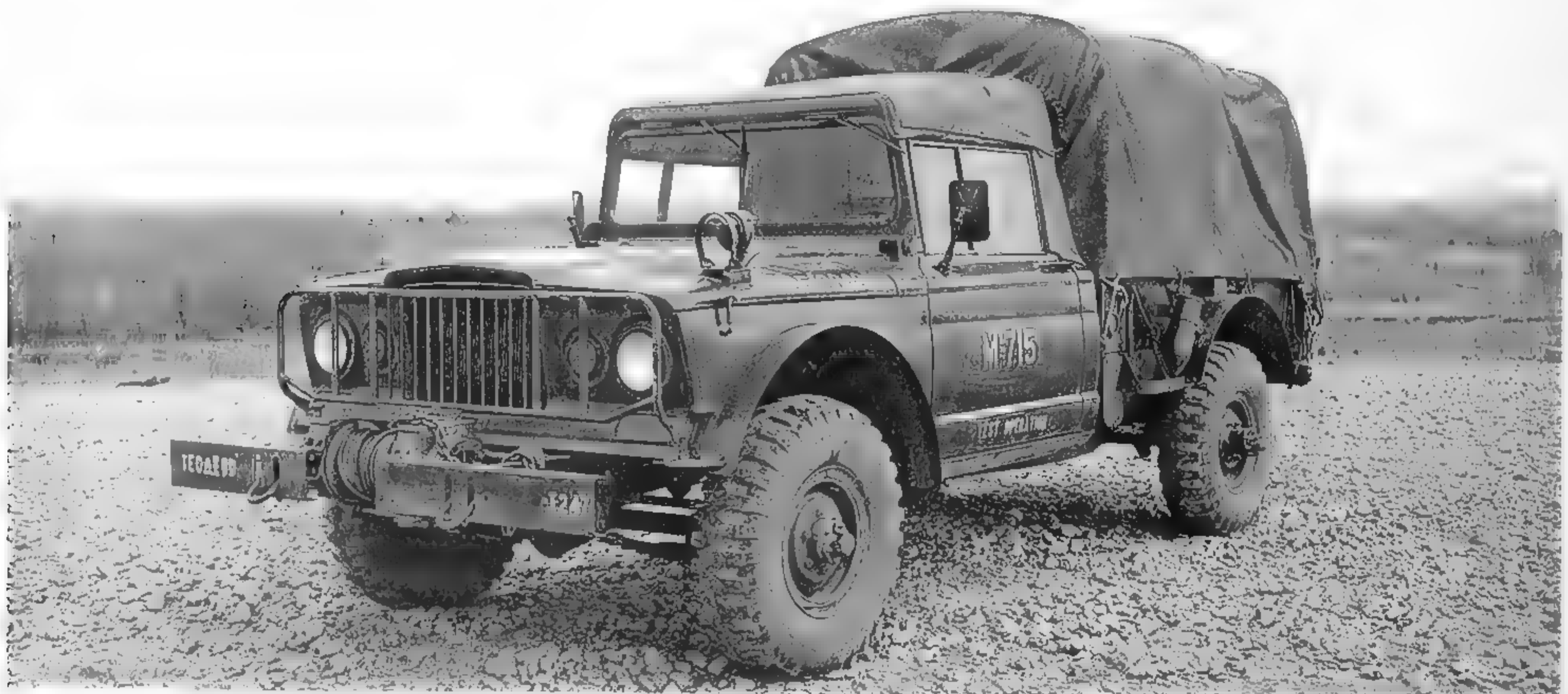
This is an XM715 with winch shown on trial by the Armor and Engineer Board at Fort Knox in October 1966. Although mounted differently, this is the same type 7,500-lb.-capacity Braden LU-4 PTO-driven winch that was used on the G-741 series trucks, such as the M37. (Photo courtesy the Patton Museum)
